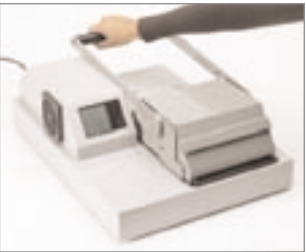
Close the flash machine and activate the flash (with most devices, the flash is automatically activated after the lid has been closed).
