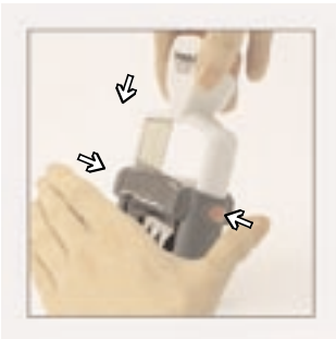
Adjusting the date bands to the exact height of the textplate:
